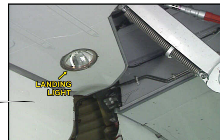
Figure 70 Landing Lights Schematic Page 140
